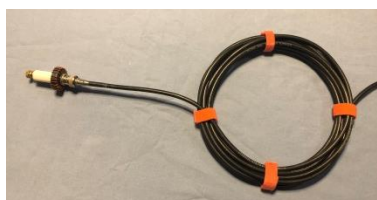
Fig 2. Scramble-wound common mode choke and transformer
