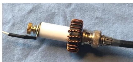
Fig 3. Spark Plug Transformer detail The EFHW wire was first tested
